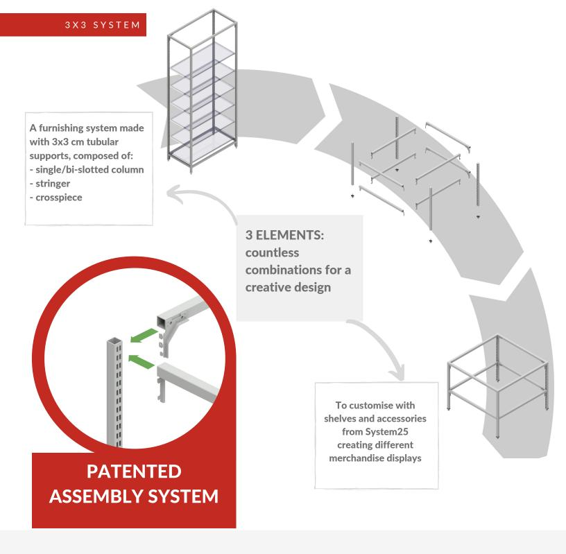
The single pieces are assembled without any type of welding or screws.
